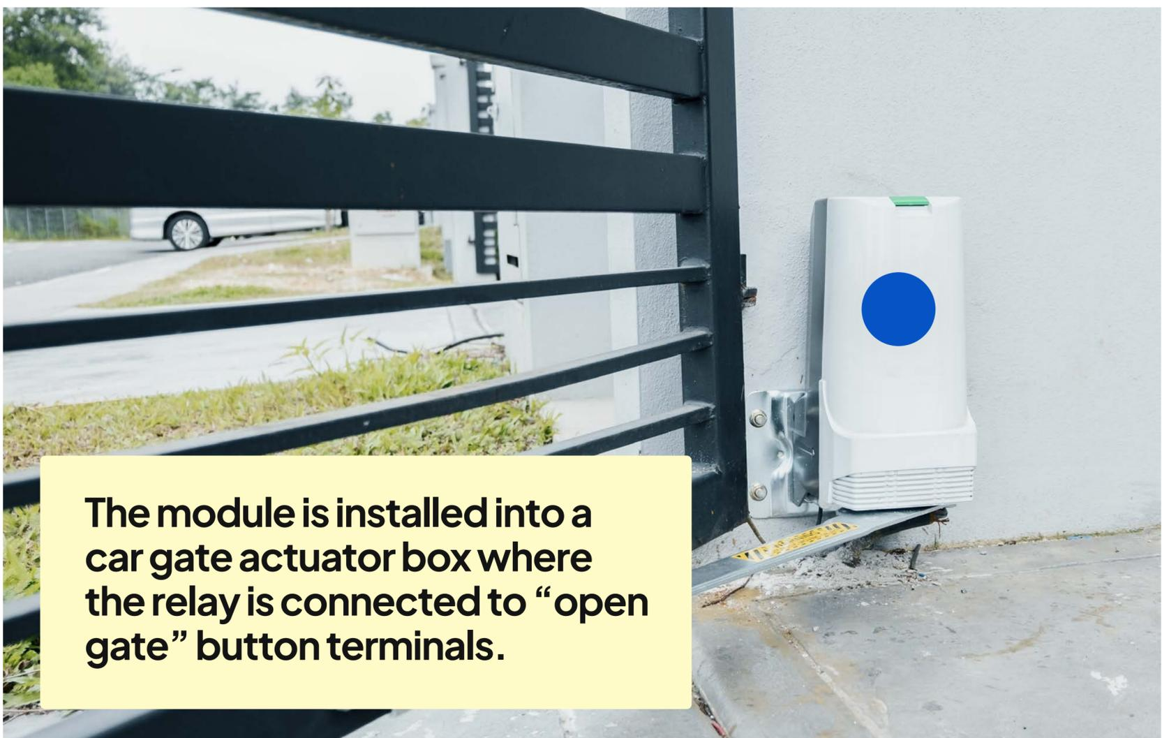
The module is installed into a car gate actuator box where the relay is connected to “open gate” button terminals.
